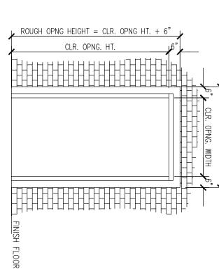
ROUGH OPENING FOR ENTRANCE INSTALLATION CMU, CONCRETE CONSTRUCTION ONLY; ROUGH OPENING IS NOT REQUIRED FOR DRY WALL CONSTRUCTION
