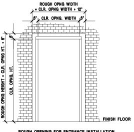
ROUGH OPENING FOR ENTRANCE INSTALLATION CMU, CONCRETE CONSTRUCTION ONLY; ROUGH OPENING IS NOT REQUIRED FOR DRY WALL CONSTRUCTION
