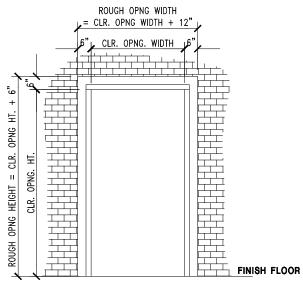
ROUGH OPENING FOR ENTRANCE INSTALLATION CMU, CONCRETE CONSTRUCTION ONLY; ROUGH OPENING IS NOT REQUIRED FOR DRY WALL CONSTRUCTION
